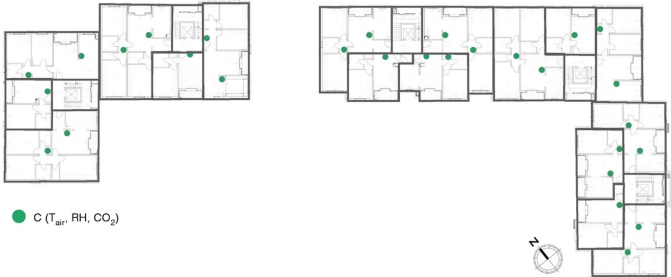
Figure 4. Air temperature sensors distribution in a floor type: one-bedroom apartments present one sensor, two or more room apartments present two sensors.
